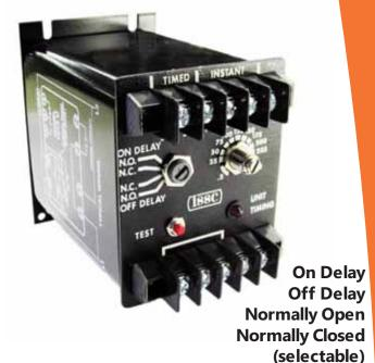
**Ease of Use Design** and selectable output makes this unit extremely flexible. This unit optically isolated control circuit operates at 120 VAC and has transient protection to 1500 volts.
