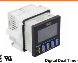
The 1096 features a large, easy to read LCD display with programmable time ranges from 0.001 seconds to 9999 hours in 6 on/off delay or repeat cycle timing functions. On time and off time are set independently. Three power supply options are available, a wide range of 100 to 240 VAC/DC, a 12 to 24VDC and a 24 VAC only version. A battery back-up maintains memory up to 7 years. Output is an SPDT relay or open collector transistor.
