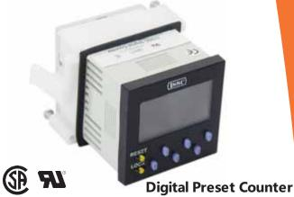
**The 1105C features** two 2 input and 5 input functions and a large, 6 digit LCD display. Two input count speeds (30/sec or 5000/sec) can be used to eliminate noise. There are 7 output functions with SPDT relay or optional transistor output. Two power supply options are available, a wide range of 100 to 240 VAC and a 12 to 24VDC only version. A battery back-up maintains memory up to 7 years.
