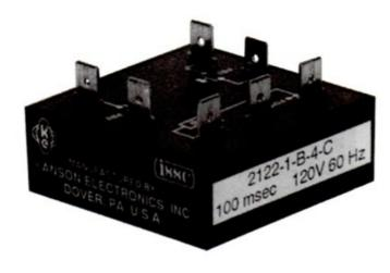
The 2122 is a compact encapsulated timer that requires inputs from two sources that must be applied within 50 msec to initiate timing sequence. If one input is held closed, closing the other input will not initiate timing cycle. The reliable, 1 Amp solid state output offers pulse widths from 50 msec to 1 second suitable for driving most valves or solenoids. Operating voltages of 24, 120 or 240 VAC.
